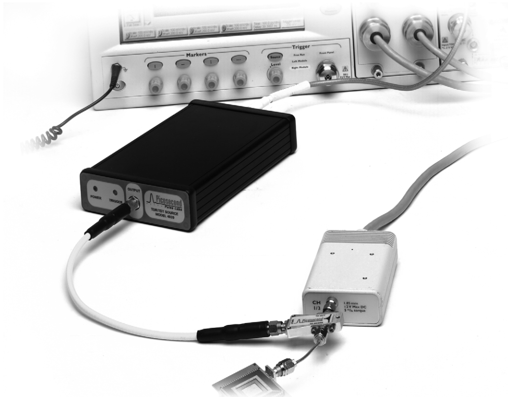
Figure 10: Picosecond Pulse Labs 4020 amplifier, microcircuit and 86118A sampler head.
